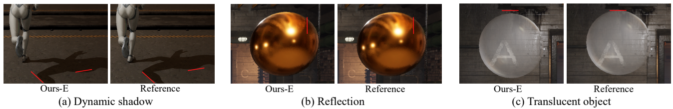
Figure 9: Example results of our extrapolation method on dynamic shadow (a), metal reflection (b), and a translucent object (c), with each compared to the reference image for clearer visibility. Our lightweight approach ignores costly shading calculations, which can cause low frame rate effects such as misaligned shadows, reflections, and translucent objects comparing with the reference (refer to red line indicators). Avoiding low frame rate inputs before frame generation can mitigate these issues. We recommend an input frame rate greater than 30 fps.
